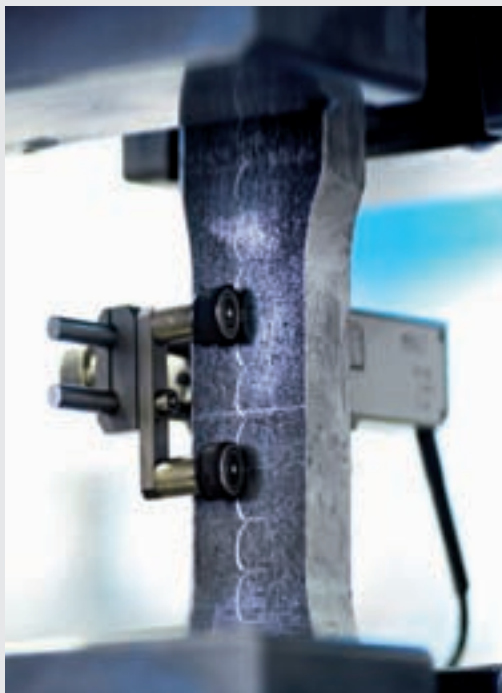
Strength determination by means of the tensile test in accordance with ASTM A 370
