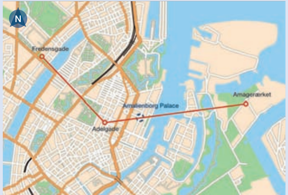
The pipeline route, at depths of up to 40.0 m, leads from the Amager peninsula off the coast under Amalienborg Palace to the »Adelgade« tunnel shaft and from there to the »Fredensgade« target shaft
