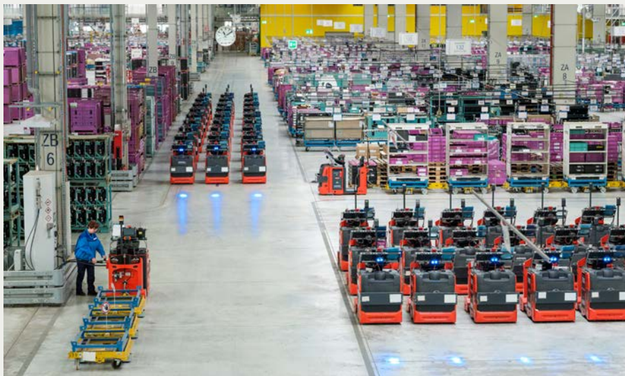
The BMW Group plant in Leipzig has been operating a large fleet of hydrogen-powered indoor factory trains since the end of 2018. These are used in production to supply the assembly lines with vendor parts.
