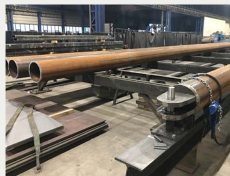
Above: At Stahl- und Anlagenbau Schädlich GmbH, the tubes were fitted with fork heads before being shot blasted and painted.
