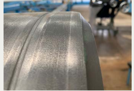
The pipes produced at Mannesmann Line Pipe's Hamm site were given a special groove and chamfer.
